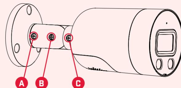
5. Tighten the adjustment screws to secure the position.
