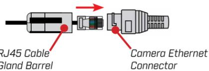
**NOTE:** The RJ45 cable gland is weather-resistant. Seal the cap with silicone and/or electrical tape for additional sealing if it will be exposed to precipitation regularly.
