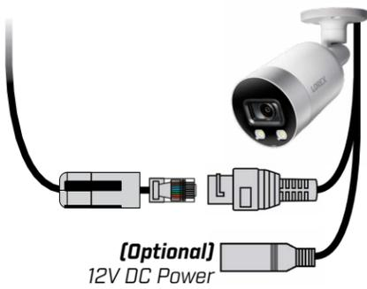
Connect the Ethernet cable to the camera.
